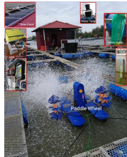
Fig. 4. Dissolved oxygen optimiser prototype in full operation due to low DO concentration
