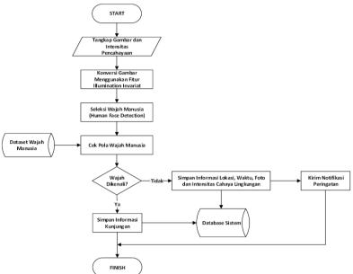
Figure 7. Detection System Flowchart.
