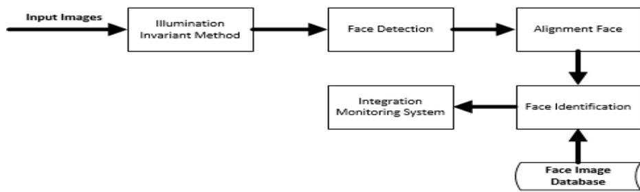
**Figure 1.** System Design Model.
