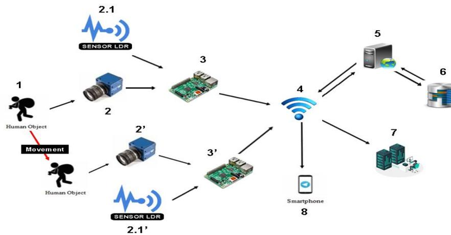
**Figure 6.** System Framework Model.
