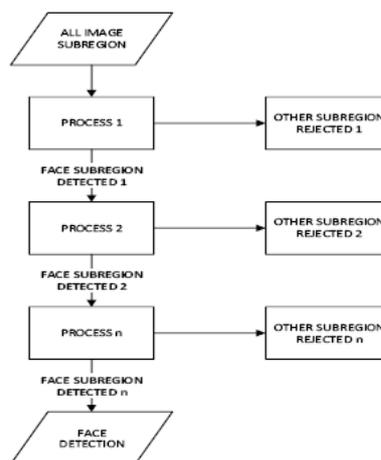
**Figure 3.** Face Detection Process.
