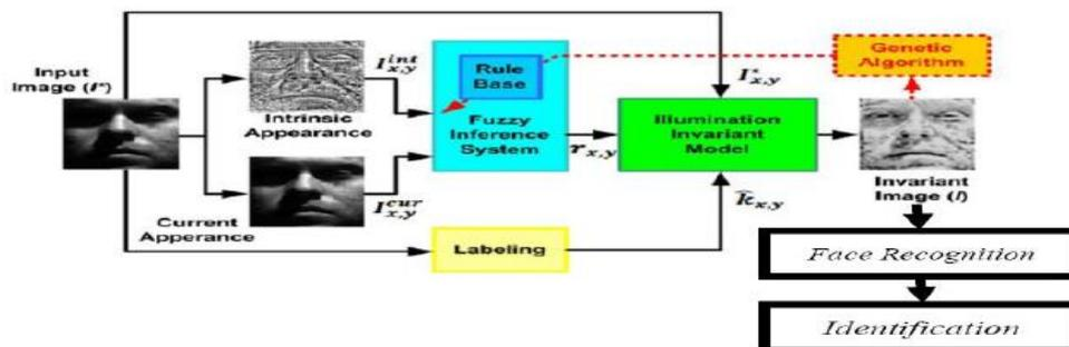
Figure 8. Illumination Invariant Identification Model.
