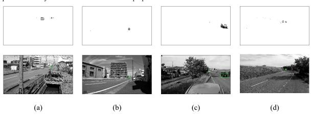
Figure 1. Sample detection of  $I_{FO}(x, y, t)$  (first row) and final result of incoming traffic detection (second row): (a) Site 2; (b) Site 4; (c) Site 7; (d) Site 12.
