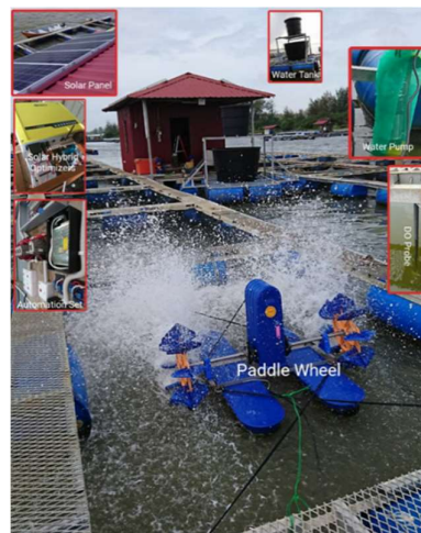
Fig. 4. Dissolved oxygen optimiser prototype in full operation due to low DO concentration
