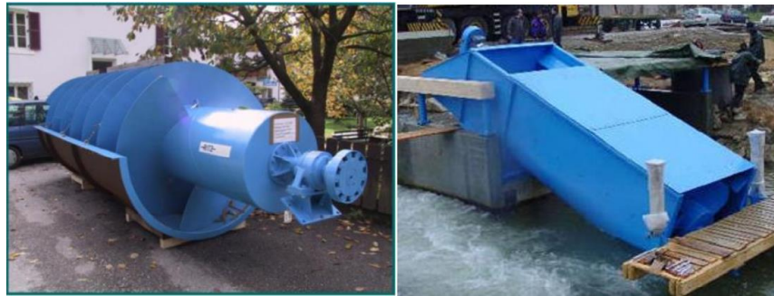
Gambar 2. Turbin Screw (a) Tipe Steel Strough dan (b) Tipe Closed Compact Installation
