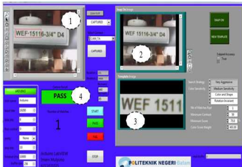
Gambar 13. Front panel pengujian program test pass
