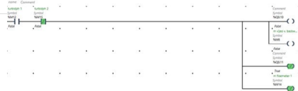
Gambar 14. Valve Backwash Close
