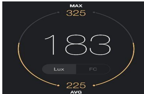
FIGURE 7. Revi room light value in lux light meter application
