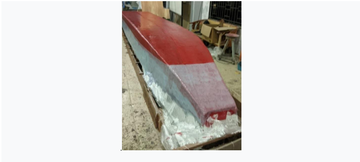
FIGURE 7.. The canoe hull lamination process uses fiberglass mixed with pigment (source: activity documentation)
