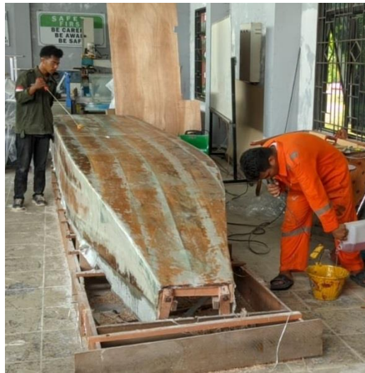
FIGURE 6. The canoe hull lamination process uses fiberglass (source: activity documentation)
