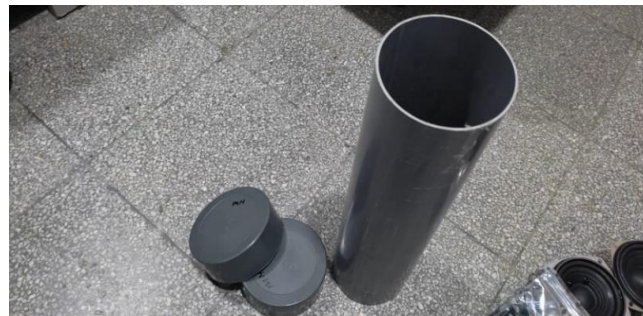
Figure 4.5 PVC Pipe as Speaker Cover
