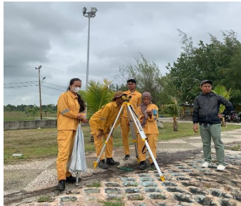
Figure 5. Seawall slope measurement
