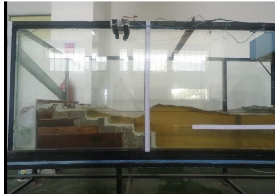
Figure 9. Seawall prototype testing in a wave flume
