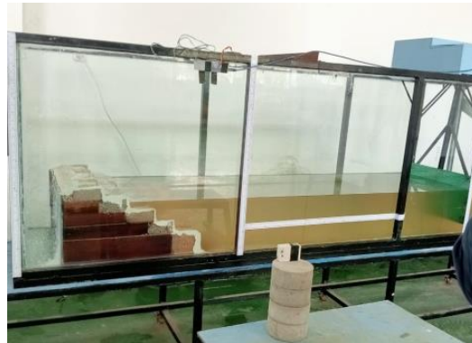
Figure 7. Wave test flume and Stepped seawall prototype
