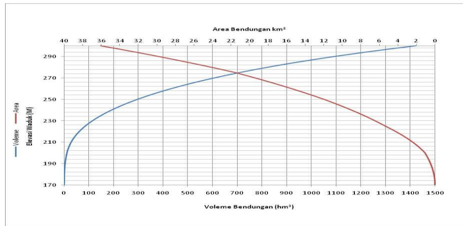
Figure 5. Graph of the relationship between elevation, volume and inundation area of Way Sekampung Reservoir Source PUPR Work Unit and O&M PSDA BBWS Mesuji Sekampung
